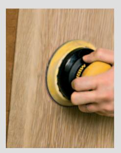
**HAZARDOUS DUST.** Sanding dust can contain harmful particles. The latest research shows that sanding hard wood is more dangerous than sanding soft wood.
