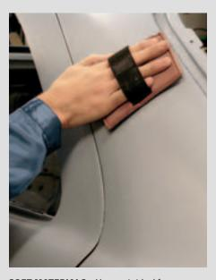
**SOFT MATERIALS.** Abranet is ideal for sanding soft materials as the anti-clogging capability will prevent the abrasive from rapid wear / premature wear compared to using traditional abrasives.
